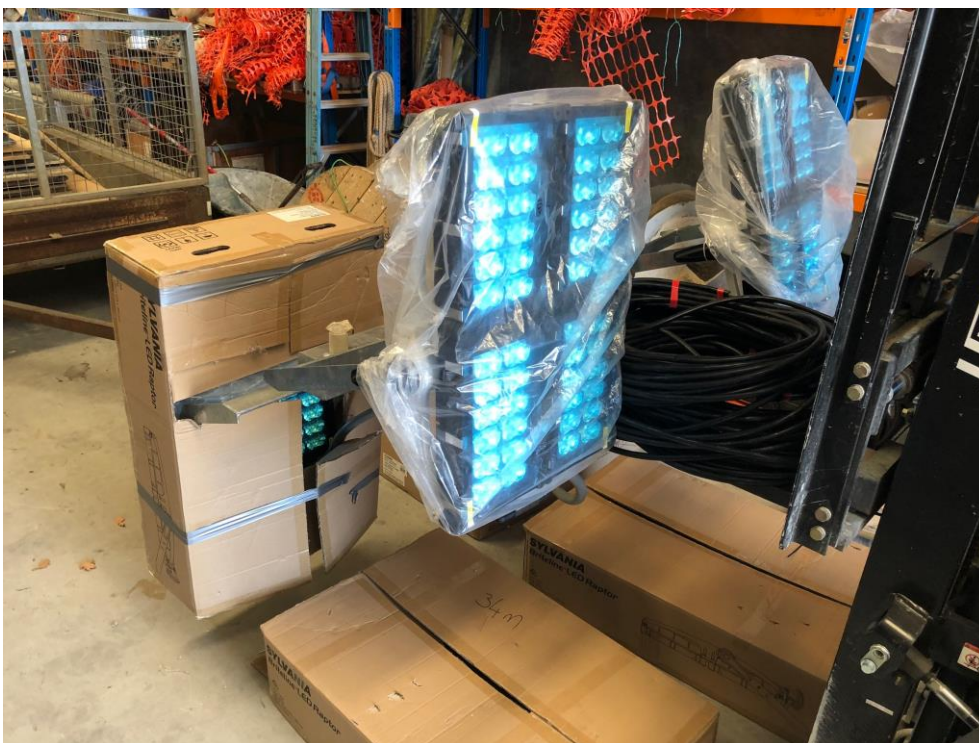
Headframe with 4no Raptor LED fittings pre-wired and mounted ready for installation
