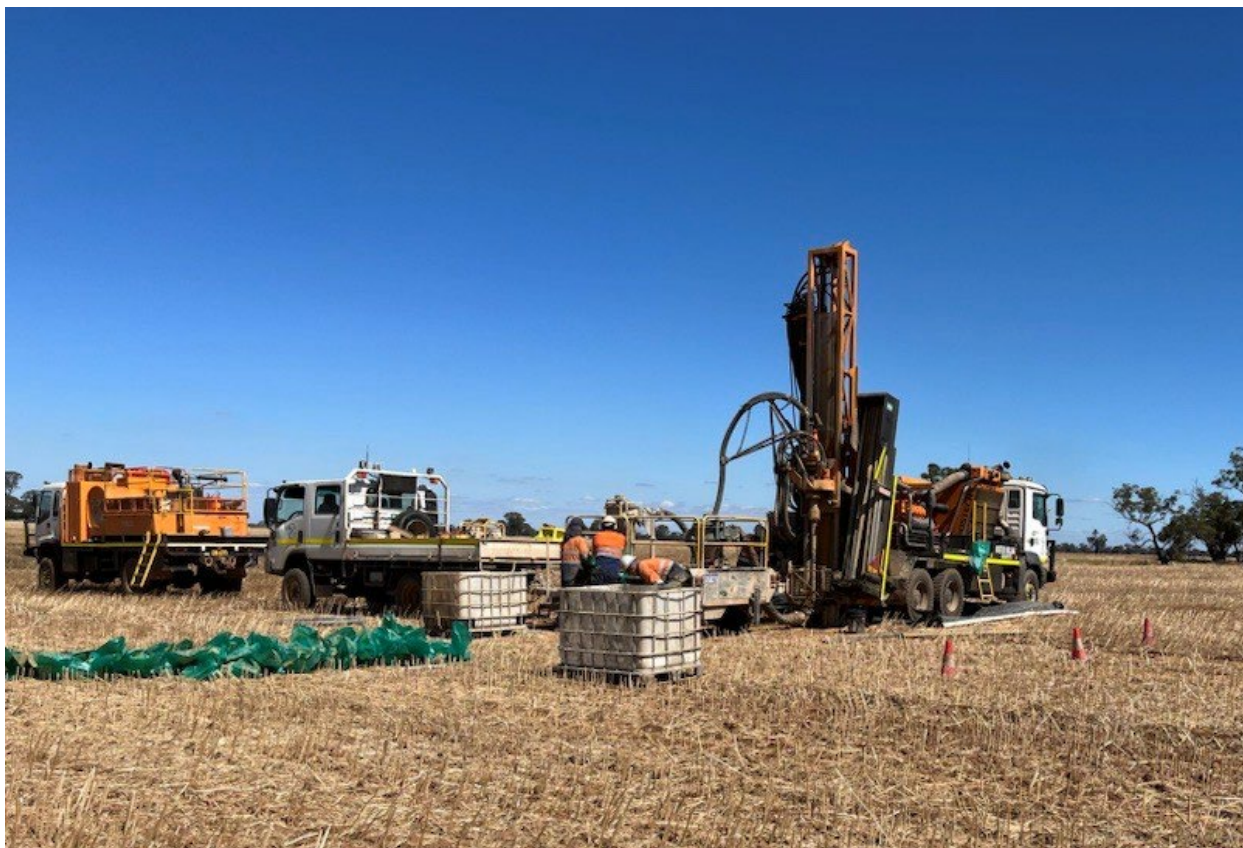
Figure 3: Aircore Drill Site showing Drill Rig, Support Vehicles and Bagged Samples
