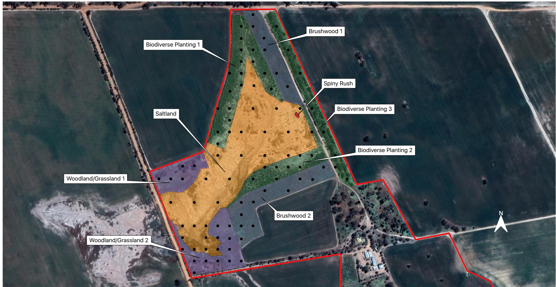
Figure 17: Proposed soil sampling sites to test soil type, pH and salinity throughout the Rehabilitation Management Area. The information from the soil sampling will be used to create a soil map and to monitor changes in salinity and pH over time. This information will help inform the choice of vegetation species to plant in different areas as the project progresses and monitor the progress of the rehabilitation project in reducing salinity and normalising soil pH over time (Base image source: Google Satellite).
