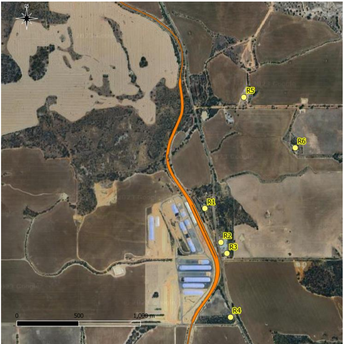
Figure 11 Proposed Rail Noise Emissions – Day Period, SPP5.4 L_{Aeq,day} (Outside the orange area is compliant)
