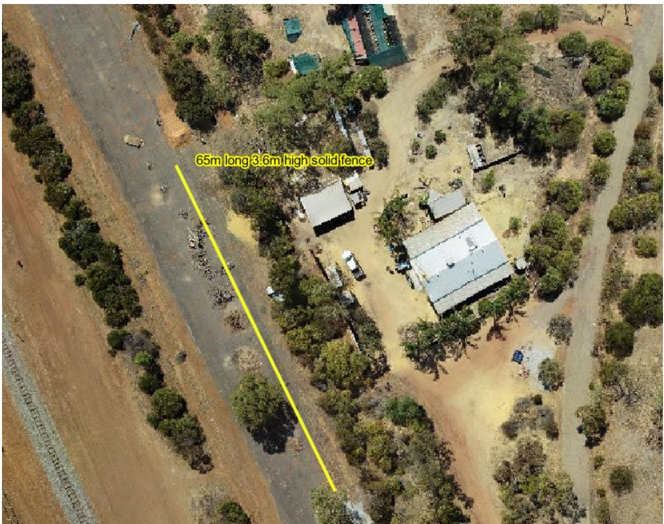
Figure 9 Receptor R1 showing proposed acoustic barrier fence on PTA land
